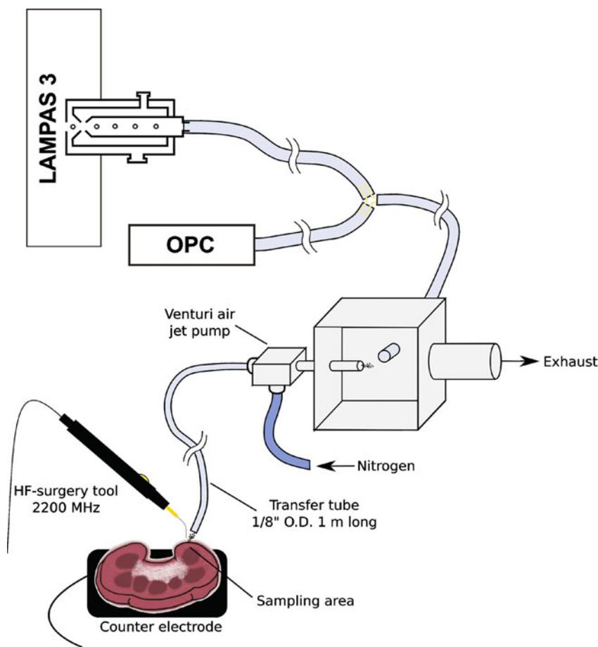
Typically, a nitrogen flow of 20 L/min was used for the operation of the Venturi pump. The electrosurgical unit was used in monopolar cutting mode with a power output of 60 W maximum.
